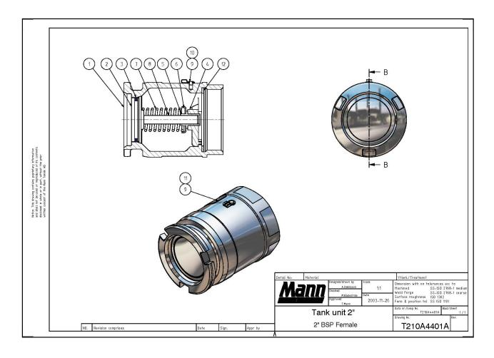
PARTS NEEDED FOR SERVICE: Spare part kit and O-ring kit (see p.3) MATERIAL: Aluminum, Brass, Stainless Steel
